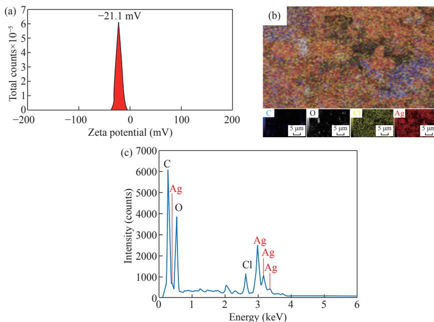
**Fig. 4** (a) Zeta potential; (b) EDS mapping; (c) EDX spectrum of Ag/AgCl synthesized at the optimal conditions
