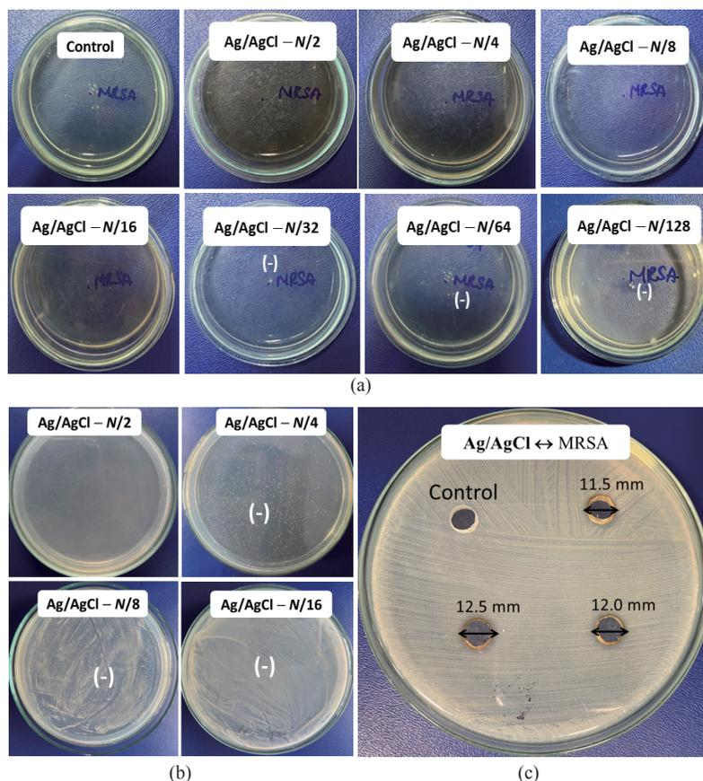
**Fig. 6** Images of (a) the minimum inhibitory concentration; (b) the minimum bactericidal concentration; (c) and the inhibition zone of Ag/AgCl nanocomposite ( $N = 132.2$  mg/L) against MRSA
