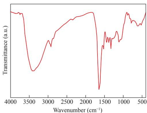
**Fig. 5** FT-IR spectrum of powder Ag/AgCl synthesized at the optimal conditions and then dried at 60  $^{\circ}\text{C}$  for 24 h
