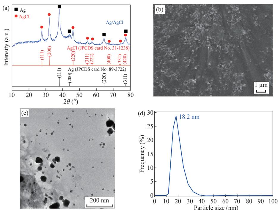
**Fig. 3** (a) XRD pattern; (b) SEM image; (c) TEM image; (d) Size distribution of Ag/AgCl synthesized at the optimal conditions
