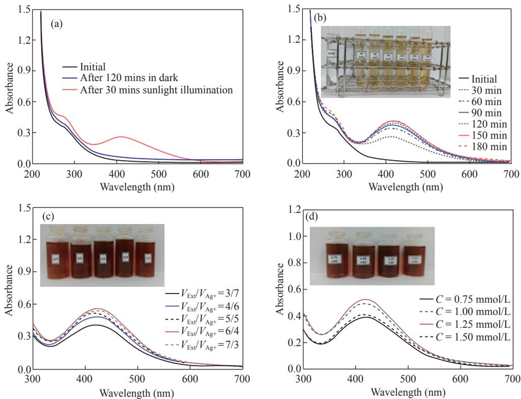
**Fig. 2** UV-Vis spectra of Ag/AgCl solutions under various conditions. (a) Effect of light illumination; (b) Synthesis duration; (c)  $V_{Ext}/V_{Ag^+}$  volume ratio; (d)  $AgNO_3$  concentration
