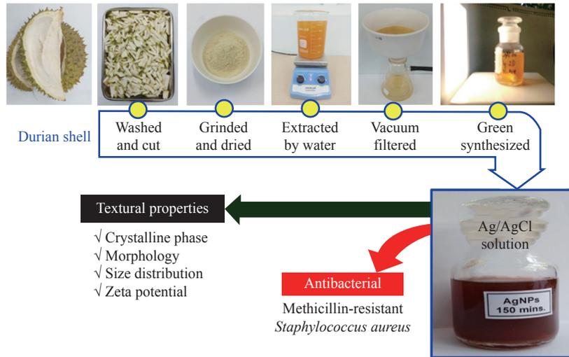
**Fig. 1** Schematic illustration of the experimental process
