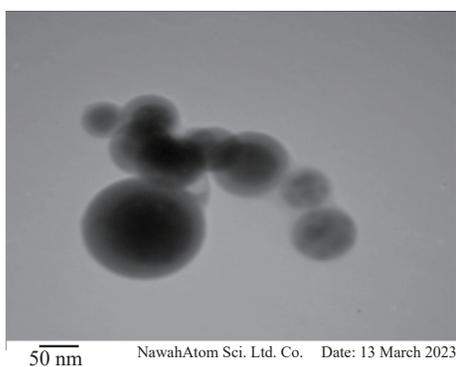
**Fig. 6** TEM image of CS-Ag nanoparticles.
