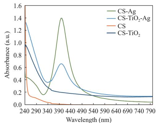
**Fig. 3** UV-Vis spectra of CS-Ag, CS-TiO<sub>2</sub>, CS-TiO<sub>2</sub>-Ag, and CS.
