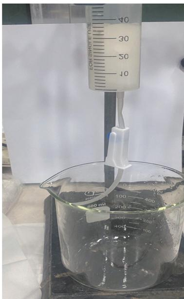
**Fig. 2** Water-purifying filter.
