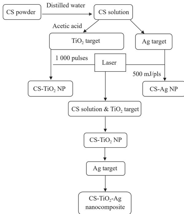
**Fig. 1** Mechanism underlying the formation of the nanocomposite (CS-TiO<sub>2</sub>-Ag).
