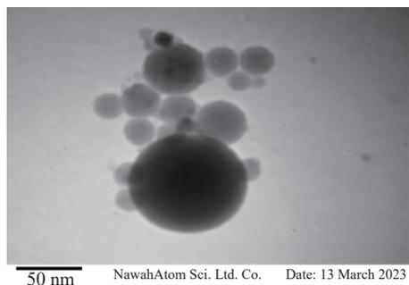
Fig. 10 TEM image of CS-TiO<sub>2</sub>-Ag nanoparticles.
