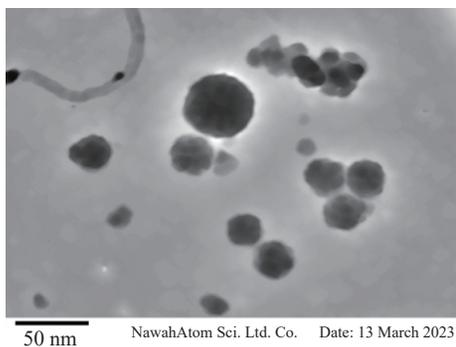
**Fig. 4** TEM image of CS nanoparticles.
