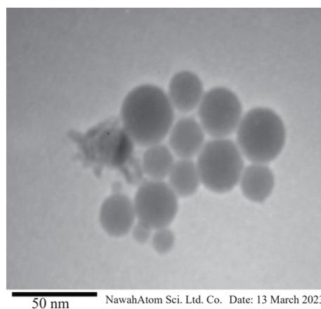
**Fig. 8** TEM image of CS-TiO<sub>2</sub> nanoparticles.
