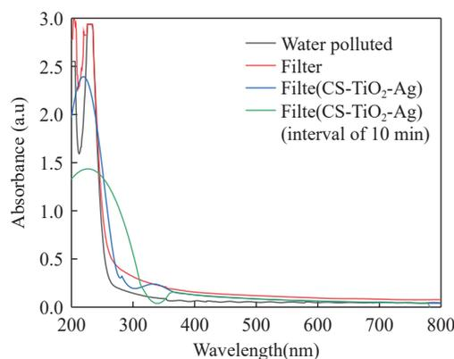
Fig. 14 UV-Vis spectra of the polluted water, sponge filter only, and sponge filter with the CS-TiO<sub>2</sub>-Ag nanocomposite.
