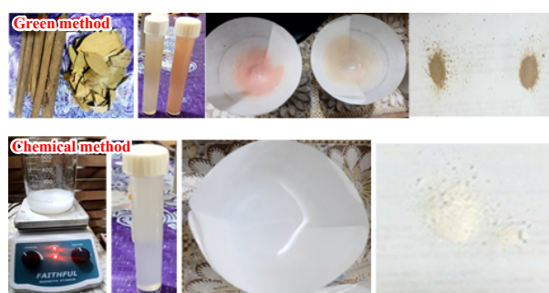
Fig. 1 Steps of the preparation process of ZnO NPs using chemical and environment-friendly methods.
