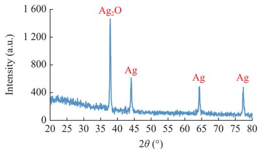
Fig. 3 XRD pattern of Ag<sub>2</sub>O nanostructure.
