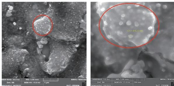
Fig. 4 SEM images of Ag<sub>2</sub>O thin film.
