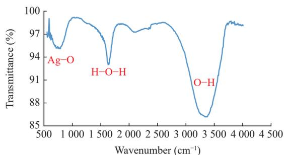
Fig. 6 FTIR spectra of  $\text{Ag}_2\text{O}$  NPs.
