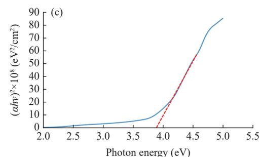
Fig. 5 (a) Absorption spectrum of Ag<sub>2</sub>O NPs. (b) Oscillating dipoles induced by light radiation of the Ag<sub>2</sub>O NPs. (c) Graph of  $(ahv)^2$  vs. photon energy  $(hv)$ .
