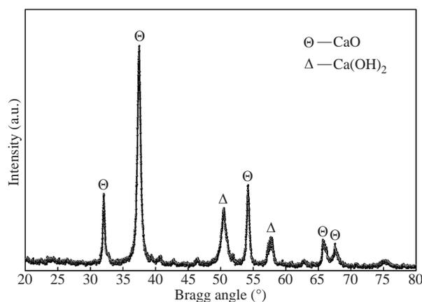
Fig. 3 XRD spectrum of CaO nanoparticles.
